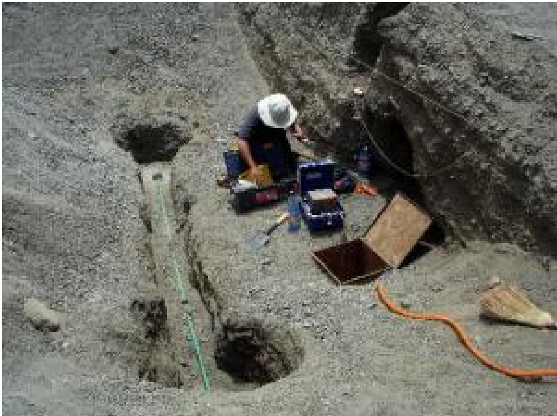
Installation of a Creepmeter of the Plate-Boundary Observatory Chile, which measures a hundredth millimeter of tektonic motions along a fault zone. (Credit: Copyright GFZ)
