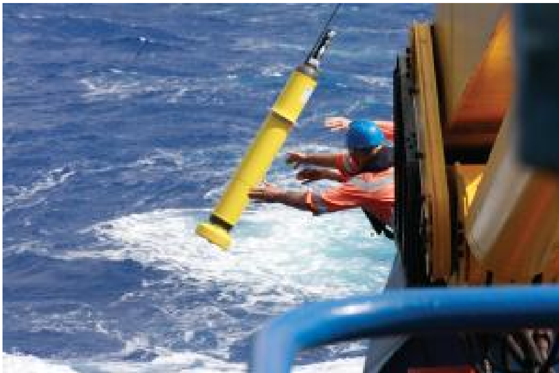
Deploying an Argo ocean profiler in the Southern Ocean. (Credit: Alicia Navidad)
